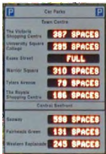
Figure 4.1: Existing Large VMS Sign
